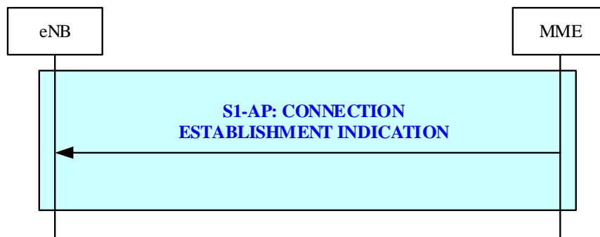
Figure 19.2.25-1: Connection Establishment Indication procedure
