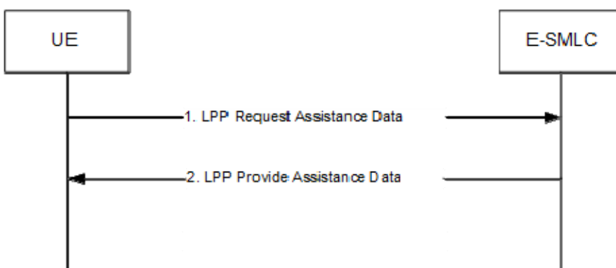
Figure 8.6.3.3.2-1: UE-initiated Assistance Data Transfer Procedure
