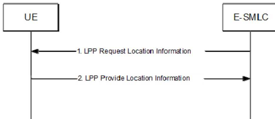
Figure 8.8.3.1.1-1: E-SMLC-initiated Location Information Transfer Procedure
