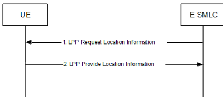
Figure 8.3.3.3.1-1: E-SMLC-initiated Location Information Transfer Procedure.
