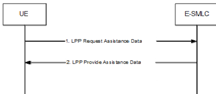
Figure 8.1.3.2.2-1: UE-initiated Assistance Data Transfer Procedure
