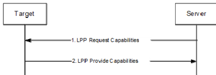
Figure 7.1.2.1-1: LPP Capability Transfer procedure
