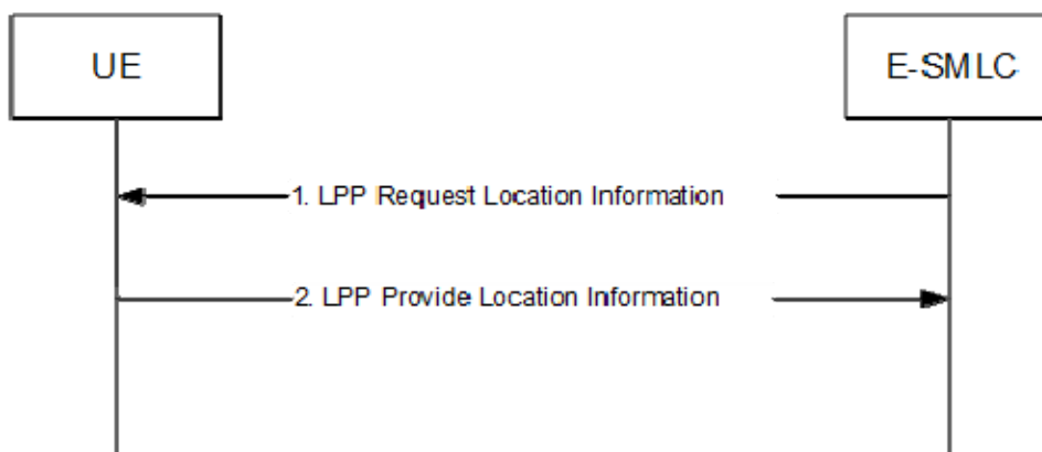
Figure 8.7.3.1.1-1: E-SMLC-initiated Location Information Transfer Procedure
