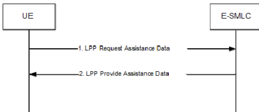
Figure 8.9.3.2.2-1: UE-initiated Assistance Data Transfer Procedure
