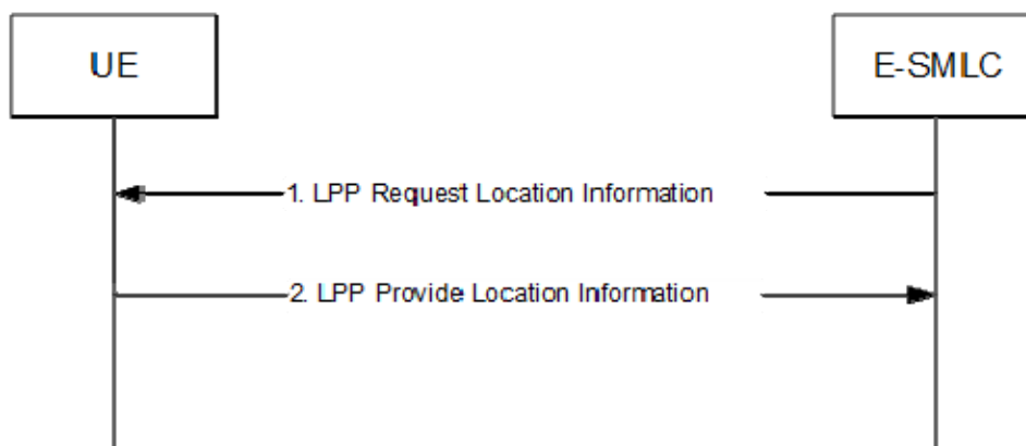
Figure 8.7.3.1.1-1: E-SMLC-initiated Location Information Transfer Procedure
