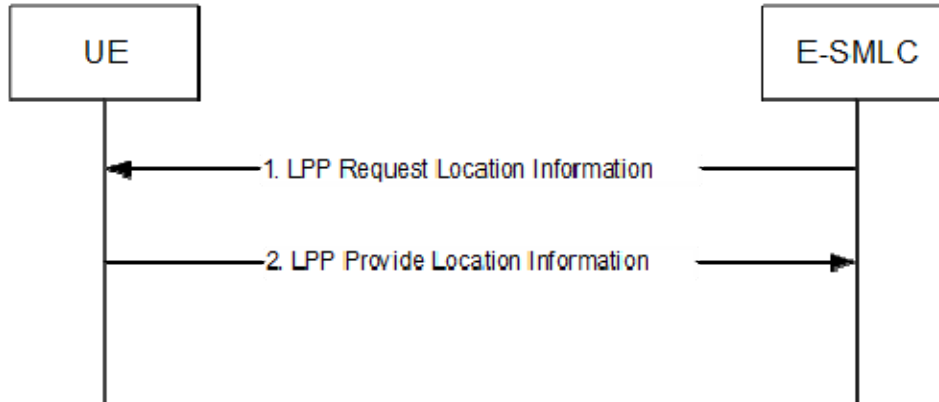
Figure 8.2.3.3.1-1: E-SMLC-initiated Location Information Transfer Procedure
