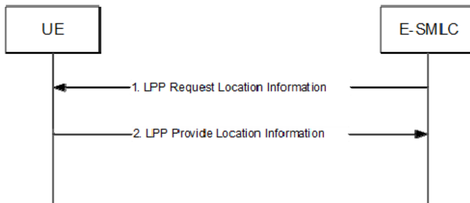
Figure 8.8.3.1.1-1: E-SMLC-initiated Location Information Transfer Procedure
