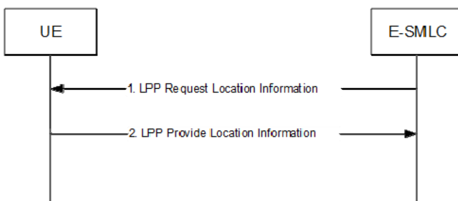
Figure 8.3.3.3.1-1: E-SMLC-initiated Location Information Transfer Procedure.
