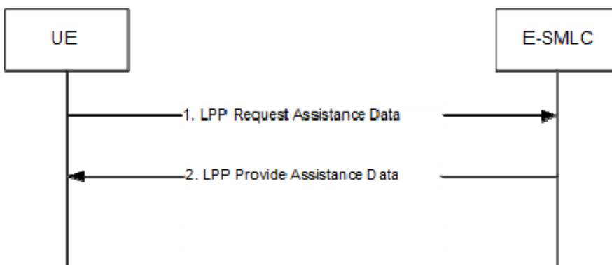
Figure 8.6.3.3.2-1: UE-initiated Assistance Data Transfer Procedure
