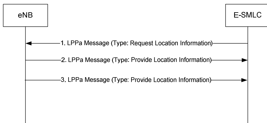
Figure 8.4.3.2-1: E-SMLC-initiated Triggered Procedure for Location Information Applicable to Downlink
