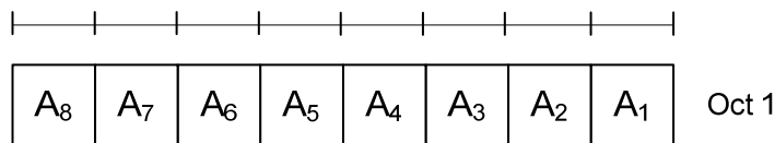
Figure 6.1.3.14-2: Activation/Deactivation CSI-RS command
