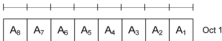
Figure 6.1.3.14-2: Activation/Deactivation CSI-RS command
