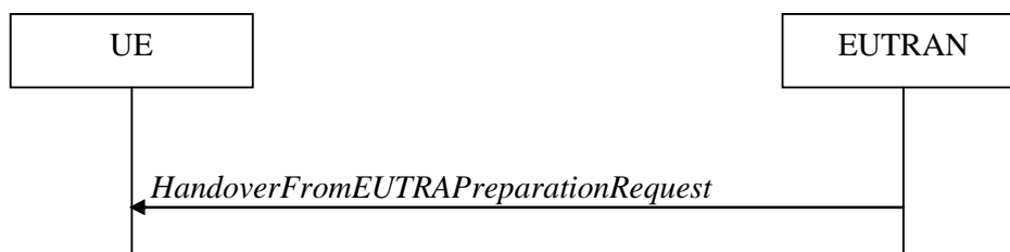
Figure 5.4.4.1-1: Handover from E-UTRA preparation request
