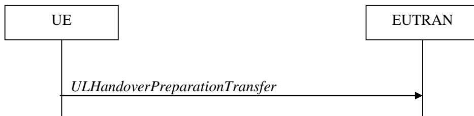
Figure 5.4.5.1-1: UL handover preparation transfer
