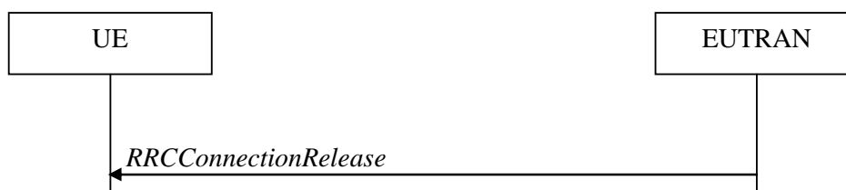
Figure 5.3.8.1-1: RRC connection release, successful
