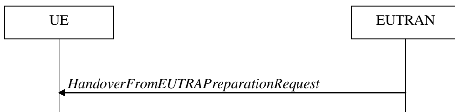
Figure 5.4.4.1-1: Handover from E-UTRA preparation request
