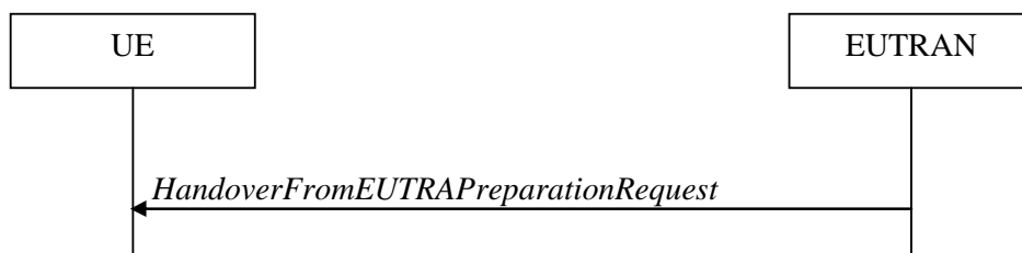
Figure 5.4.4.1-1: Handover from E-UTRA preparation request
