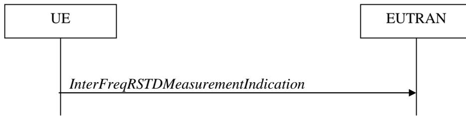
**Figure 5.5.7.1-1: Inter-frequency RSTD measurement indication**
