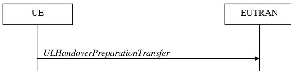
**Figure 5.4.5.1-1: UL handover preparation transfer**
