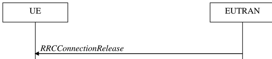
**Figure 5.3.8.1-1: RRC connection release, successful**
