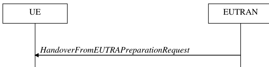
Figure 5.4.4.1-1: Handover from E-UTRA preparation request
