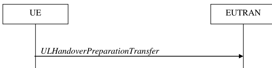
Figure 5.4.5.1-1: UL handover preparation transfer
