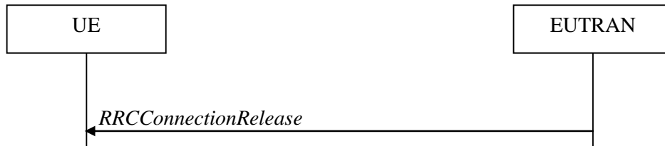
Figure 5.3.8.1-1: RRC connection release, successful
