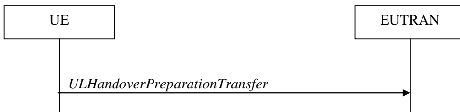
Figure 5.4.5.1-1: UL handover preparation transfer
