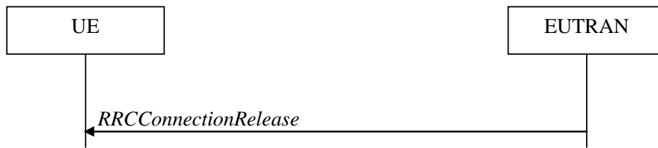
Figure 5.3.8.1-1: RRC connection release, successful
