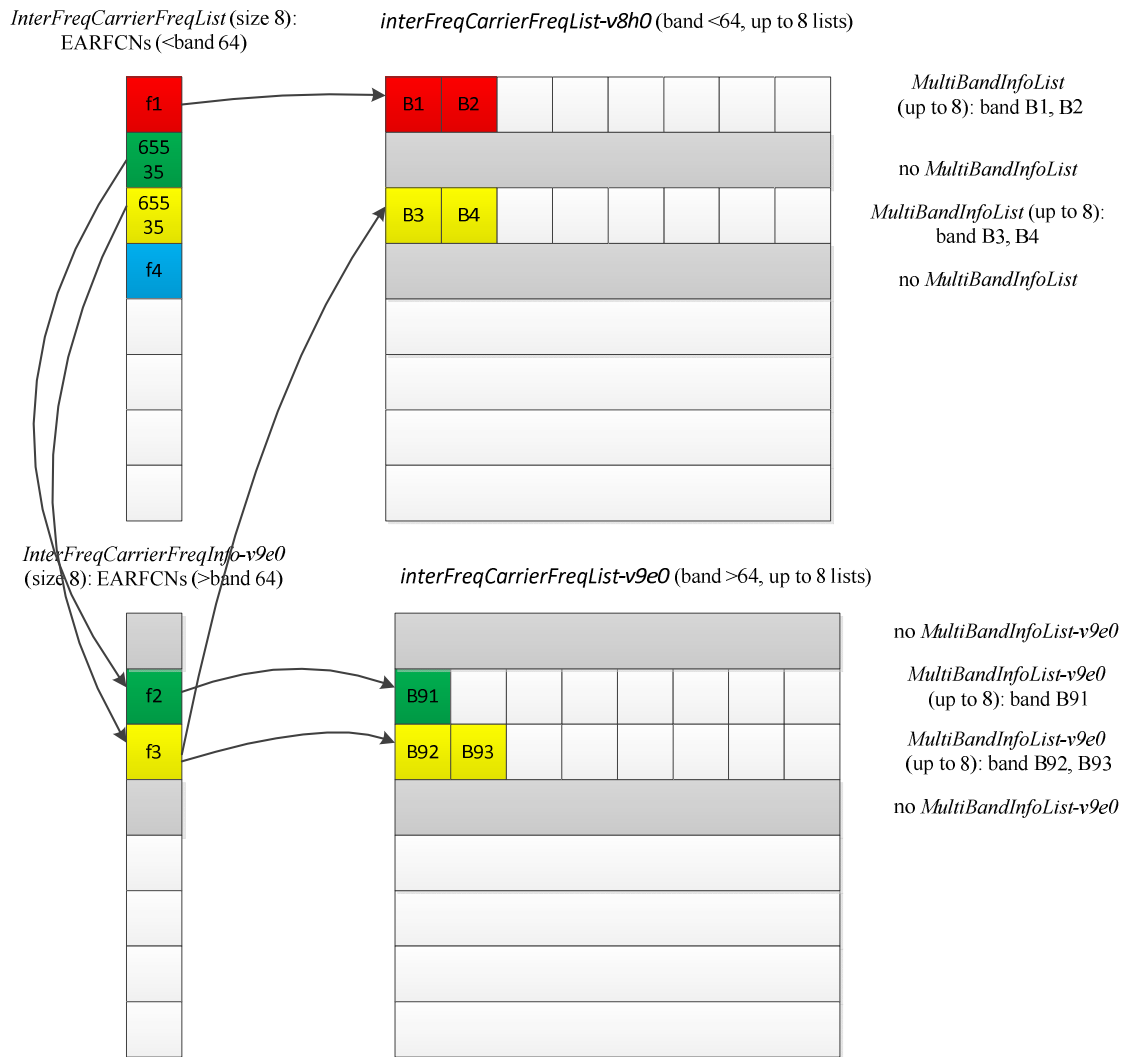
Figure D.1.2-1: Mapping of EARFCNs to MultiBandInfoList/MultiBandInfoList-v9e0
