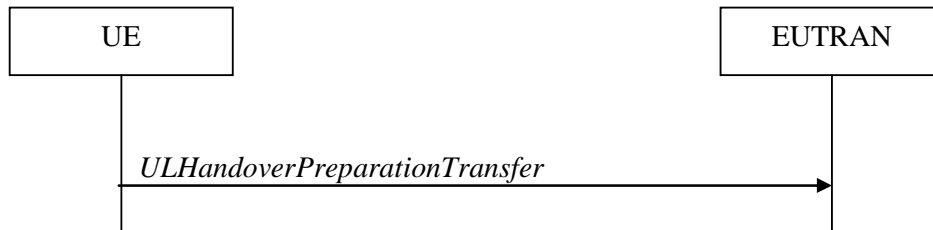
Figure 5.4.5.1-1: UL handover preparation transfer
