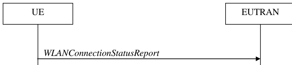
Figure 5.6.15.2.1-1: WLAN connection status reporting
