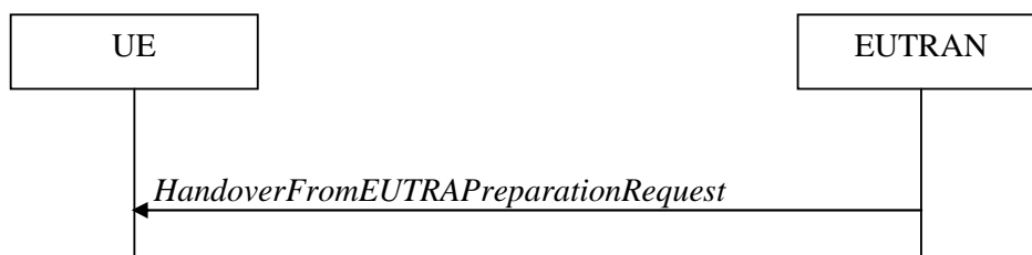
Figure 5.4.4.1-1: Handover from E-UTRA preparation request
