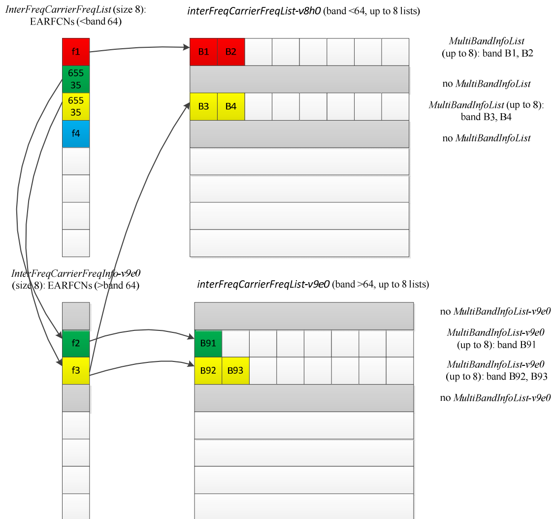
Figure D.1.2-1: Mapping of EARFCNs to MultiBandInfoList/MultiBandInfoList-v9e0
