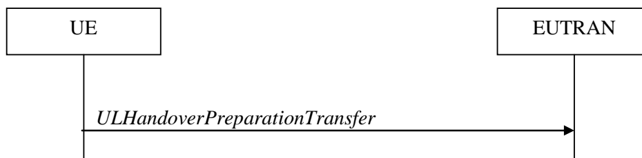
Figure 5.4.5.1-1: UL handover preparation transfer
