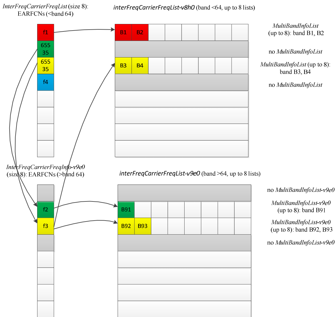
Figure D.1.2-1: Mapping of EARFCNs to MultiBandInfoList/MultiBandInfoList-v9e0
