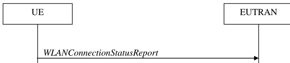
Figure 5.6.15.2.1-1: WLAN connection status reporting
