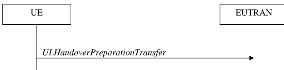
Figure 5.4.5.1-1: UL handover preparation transfer
