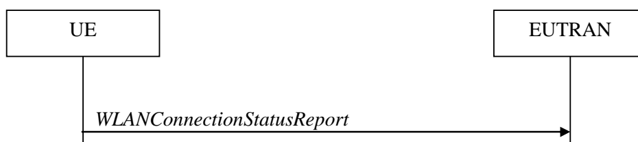
Figure 5.6.15.2.1-1: WLAN connection status reporting
