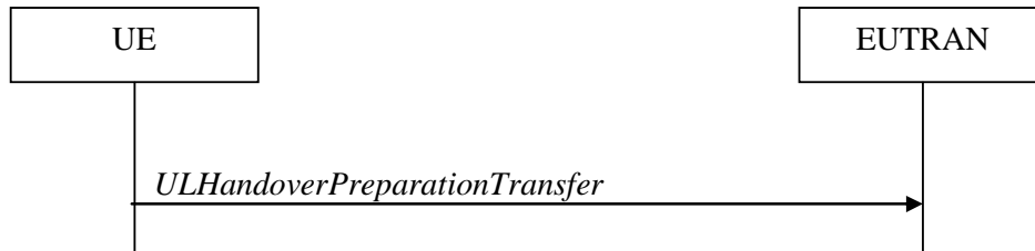
Figure 5.4.5.1-1: UL handover preparation transfer
