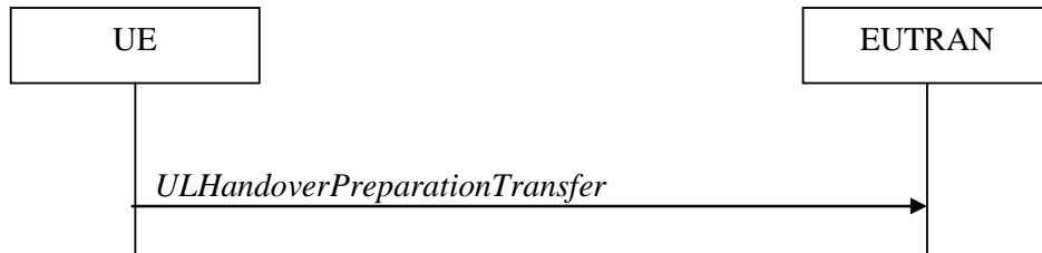
Figure 5.4.5.1-1: UL handover preparation transfer
