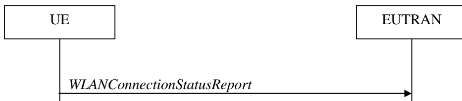
Figure 5.6.15.2.1-1: WLAN connection status reporting
