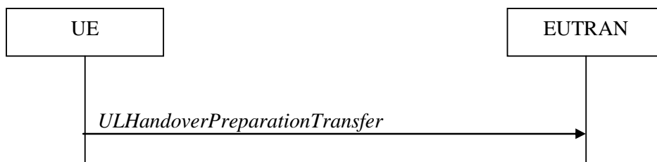
Figure 5.4.5.1-1: UL handover preparation transfer
