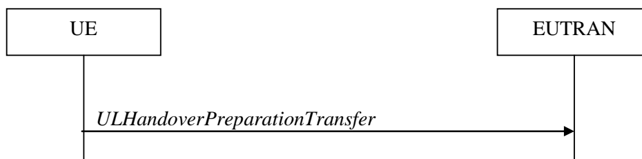
Figure 5.4.5.1-1: UL handover preparation transfer
