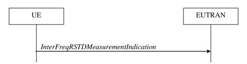
Figure 5.5.7.1-1: Inter-frequency RSTD measurement indication
