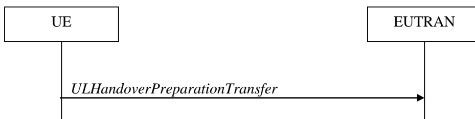
Figure 5.4.5.1-1: UL handover preparation transfer
