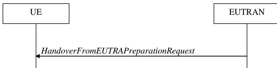
Figure 5.4.4.1-1: Handover from E-UTRA preparation request
