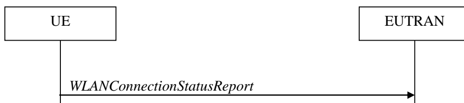
Figure 5.6.15.2.1-1: WLAN connection status reporting
