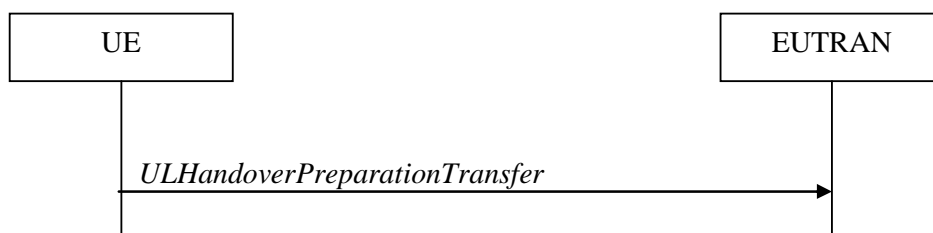
Figure 5.4.5.1-1: UL handover preparation transfer
