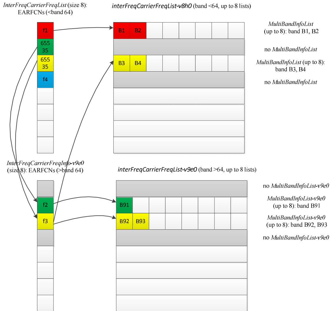
Figure D.1.2-1: Mapping of EARFCNs to MultiBandInfoList/MultiBandInfoList-v9e0
