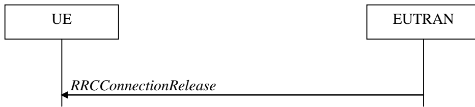
Figure 5.3.8.1-1: RRC connection release, successful
