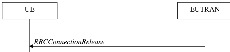
Figure 5.3.8.1-1: RRC connection release, successful
