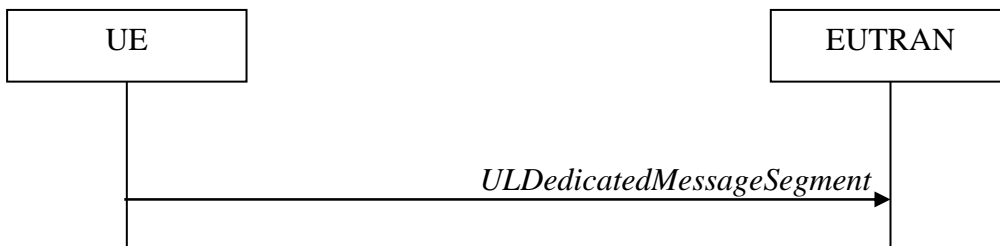
Figure 5.6.22.1-1: UL message segment transfer
