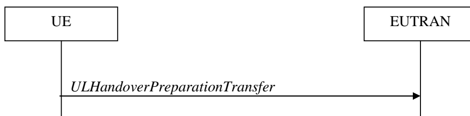
Figure 5.4.5.1-1: UL handover preparation transfer
