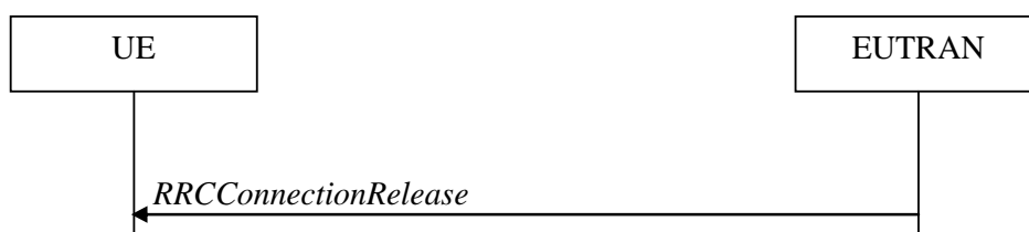
Figure 5.3.8.1-1: RRC connection release, successful
