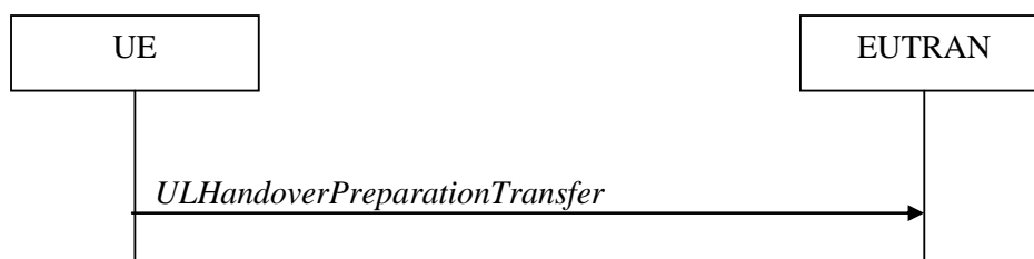
Figure 5.4.5.1-1: UL handover preparation transfer
