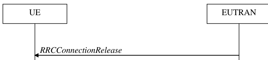
Figure 5.3.8.1-1: RRC connection release, successful
