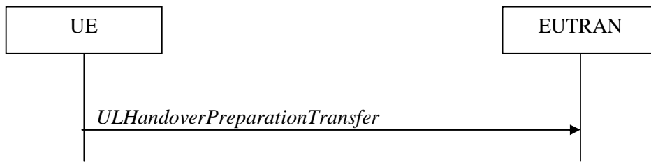
Figure 5.4.5.1-1: UL handover preparation transfer
