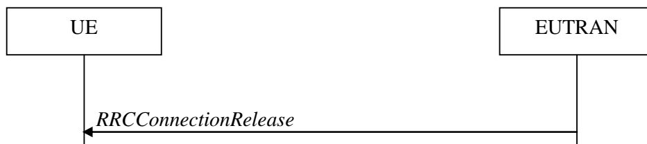
Figure 5.3.8.1-1: RRC connection release, successful
