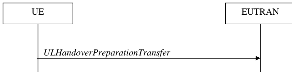
Figure 5.4.5.1-1: UL handover preparation transfer
