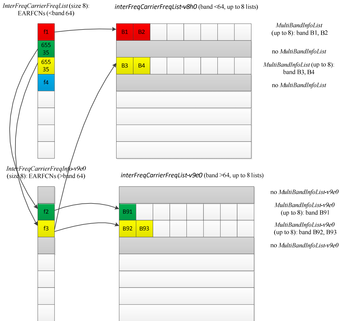
Figure D.1.2-1: Mapping of EARFCNs to MultiBandInfoList/MultiBandInfoList-v9e0
