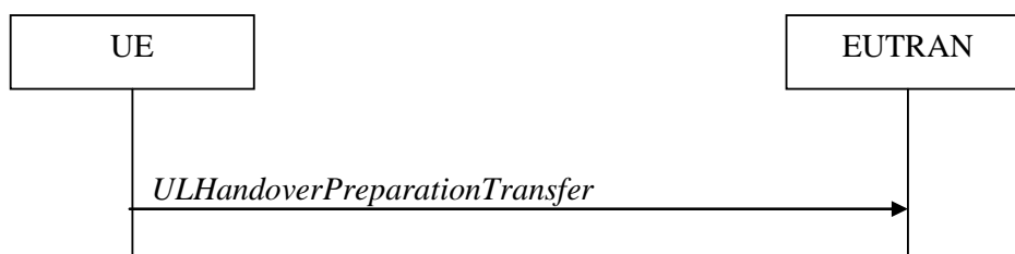
Figure 5.4.5.1-1: UL handover preparation transfer
