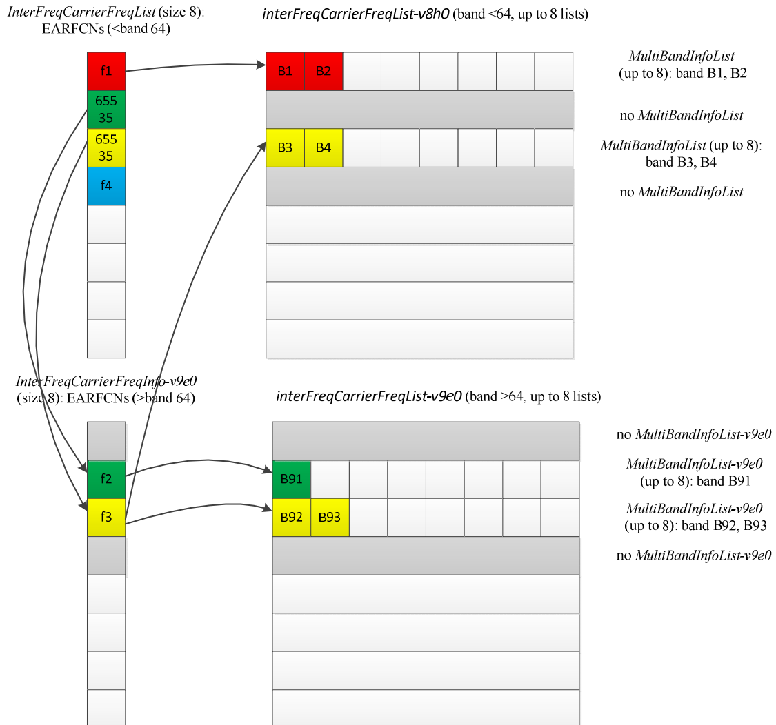
Figure D.1.2-1: Mapping of EARFCNs to MultiBandInfoList/MultiBandInfoList-v9e0
