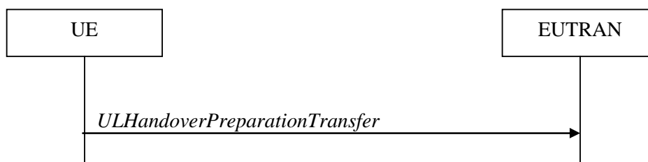
Figure 5.4.5.1-1: UL handover preparation transfer
