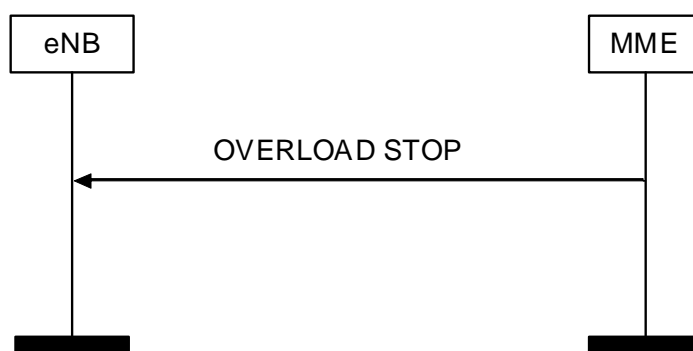
Figure 8.7.7.2.-1: Overload Stop procedure
