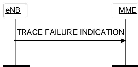
Figure 8.10.2.2-1: Trace Failure Indication procedure.
