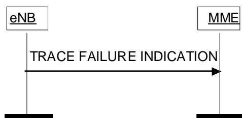
Figure 8.10.2.2-1: Trace Failure Indication procedure.
