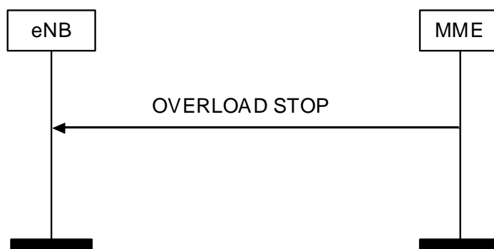
Figure 8.7.7.2-1: Overload Stop procedure
