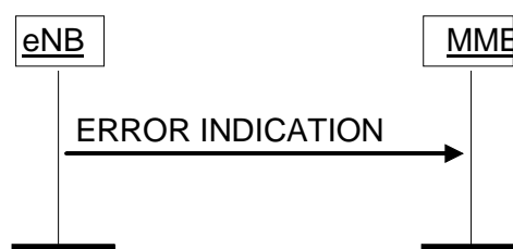
Figure 8.7.2.2-2: Error Indication procedure, eNB originated. Successful operation.
