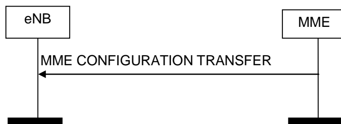
Figure 8.16.2.1-1: MME Configuration Transfer procedure. Successful operation.
