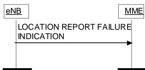
Figure 8.11.2.2-1: Location Report Failure Indication procedure.
