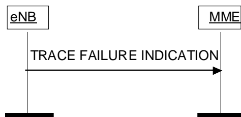
Figure 8.10.2.2-1: Trace Failure Indication procedure.
