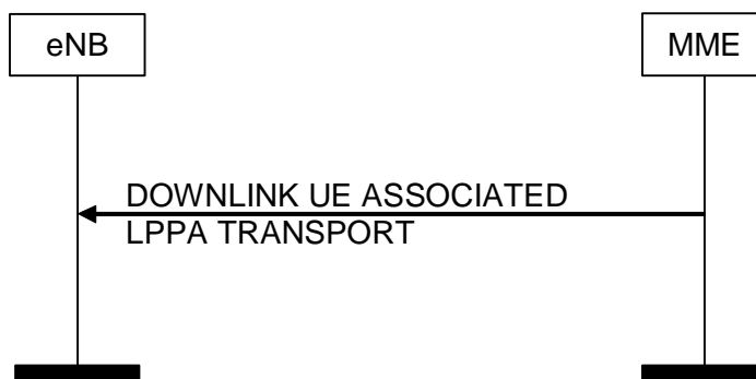
Figure 8.17.2.1-1: DOWNLINK UE ASSOCIATED LPPA Transport Procedure
