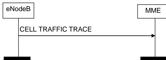
Figure 8.10.4.2-1: Cell Traffic Trace procedure. Successful operation.
