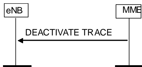
Figure 8.10.3.2-1: Deactivate Trace procedure. Successful operation.
