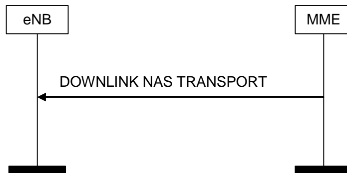
Figure 8.6.2.2-1: DOWNLINK NAS Transport Procedure
