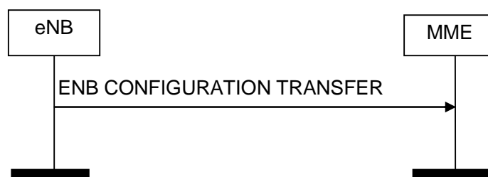
Figure 8.15.2.1-1: eNB Configuration Transfer procedure. Successful operation.
