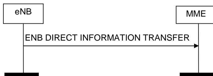
Figure 8.13.1.2-1: ENB Direct Information Transfer procedure. Successful operation.
