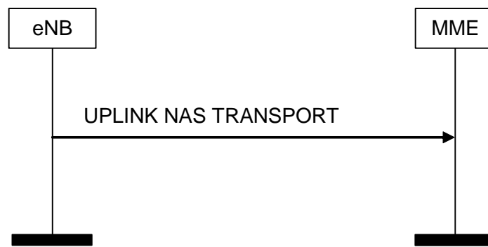
Figure 8.6.2.3-1: UPLINK NAS TRANSPORT Procedure
