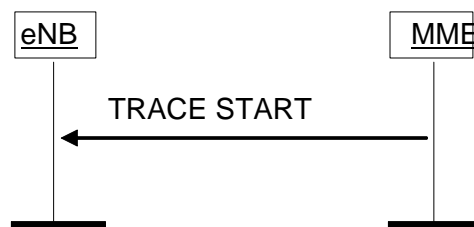
Figure 8.10.1.2-1: Trace Start procedure.
