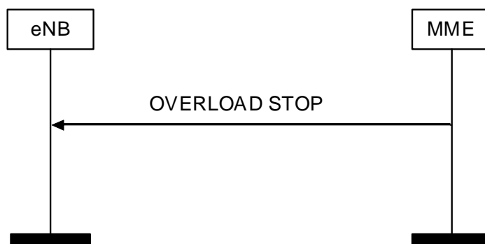
Figure 8.7.7.2.-1: Overload Stop procedure
