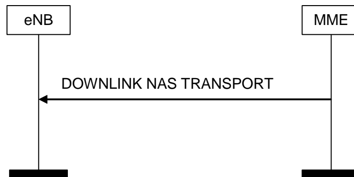
Figure 8.6.2.2-1: DOWNLINK NAS Transport Procedure
