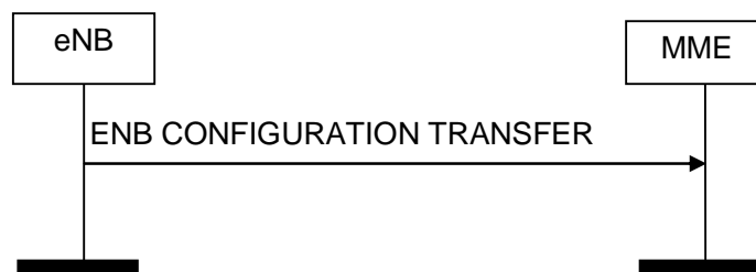
Figure 8.15.2.1-1: eNB Configuration Transfer procedure. Successful operation.
