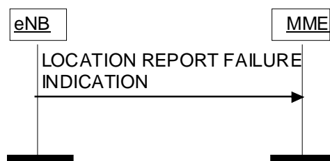
Figure 8.11.2.2-1: Location Report Failure Indication procedure.
