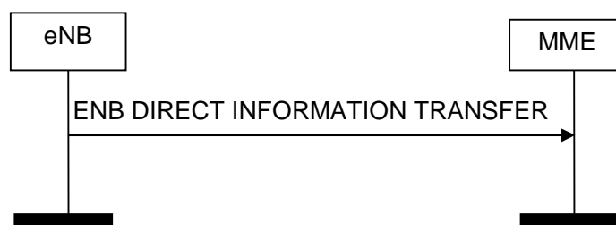
Figure 8.13.1.2-1: ENB Direct Information Transfer procedure. Successful operation.
