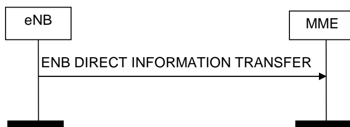
Figure 8.13.1.2-1: ENB Direct Information Transfer procedure. Successful operation.
