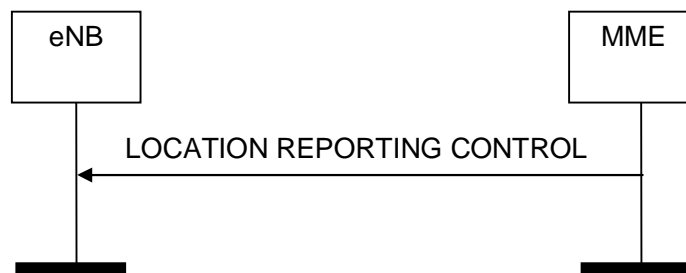
Figure 8.11.1.2-1: Location Reporting Control procedure. Successful operation.
