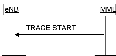
Figure 8.10.1.2-1: Trace Start procedure.
