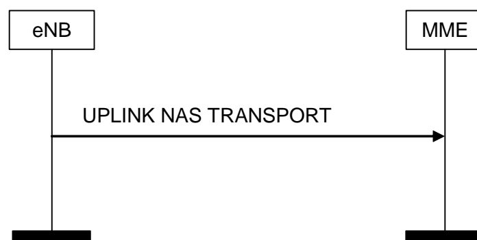
Figure 8.6.2.3-1: UPLINK NAS TRANSPORT Procedure
