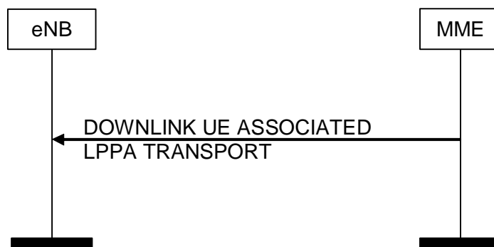
Figure 8.17.2.1-1: DOWNLINK UE ASSOCIATED LPPA Transport Procedure
