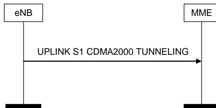
Figure 8.8.2.2-1: Uplink S1 CDMA2000 Tunneling Procedure
