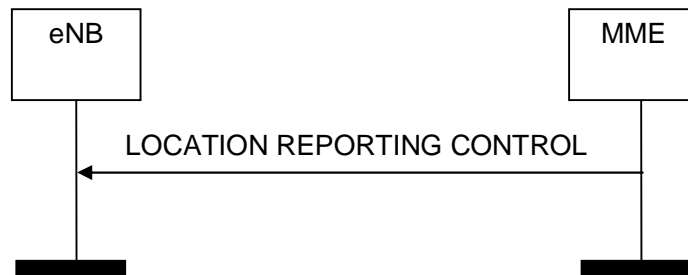
Figure 8.11.1.2-1: Location Reporting Control procedure. Successful operation.
