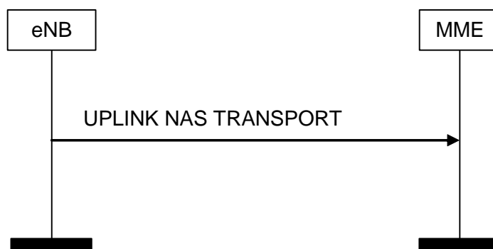
Figure 8.6.2.3-1: UPLINK NAS TRANSPORT Procedure
