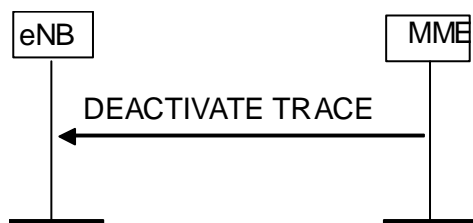
Figure 8.10.3.2-1: Deactivate Trace procedure. Successful operation.
