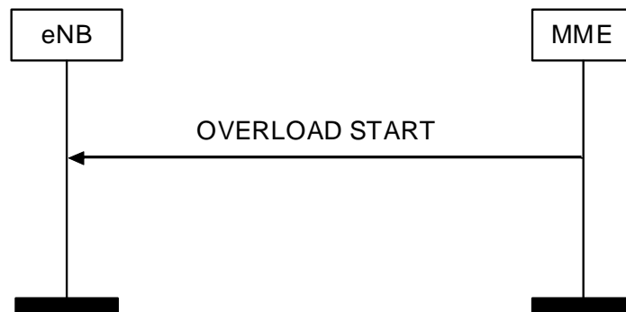
Figure 8.7.6.2-1: Overload Start procedure
