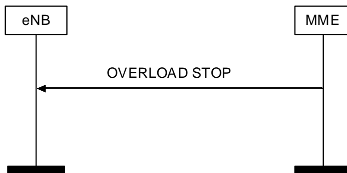
Figure 8.7.7.2.-1: Overload Stop procedure
