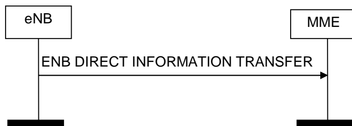
Figure 8.13.1.2-1: ENB Direct Information Transfer procedure. Successful operation.
