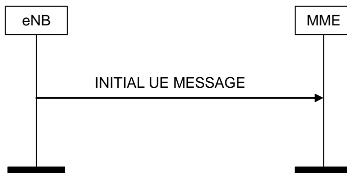
Figure 8.6.2.1-1: Initial UE Message procedure
