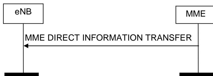
Figure 8.14.1.2-1: MME Direct Information Transfer procedure. Successful operation.
