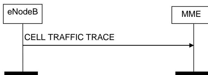
Figure 8.10.4.2-1: Cell Traffic Trace procedure. Successful operation.
