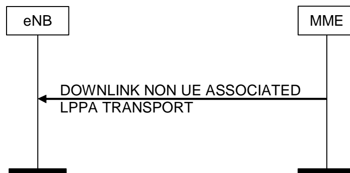
Figure 8.17.2.3-1: DOWNLINK NON UE ASSOCIATED LPPA Transport Procedure
