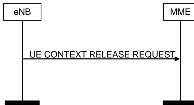
Figure 8.3.2.2-1: UE Context Release Request procedure. Successful operation.
