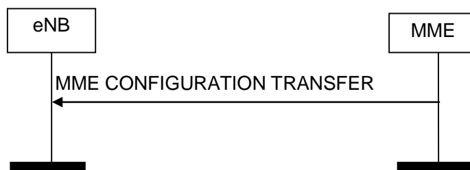
Figure 8.16.2.1-1: MME Configuration Transfer procedure. Successful operation.
