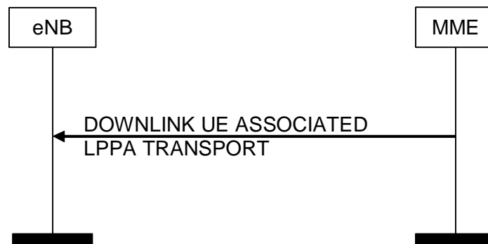
Figure 8.17.2.1-1: DOWNLINK UE ASSOCIATED LPPA Transport Procedure
