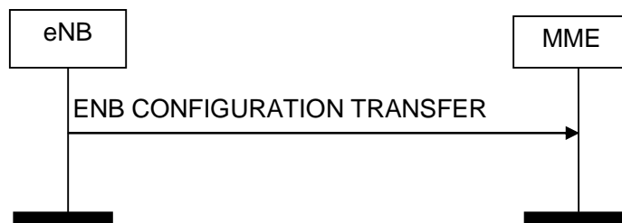
Figure 8.15.2.1-1: eNB Configuration Transfer procedure. Successful operation.
