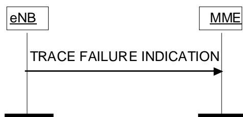
Figure 8.10.2.2-1: Trace Failure Indication procedure.
