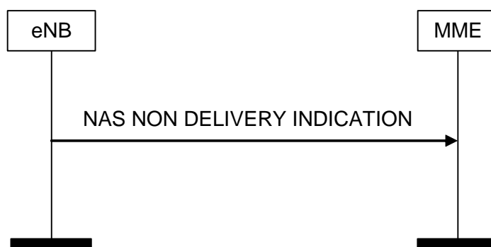
Figure 8.6.2.4-1: NAS NON DELIVERY INDICATION Procedure
