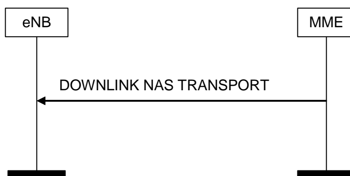
Figure 8.6.2.2-1: DOWNLINK NAS Transport Procedure
