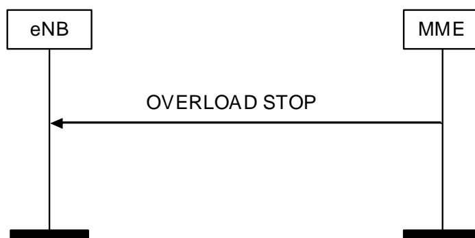
Figure 8.7.7.2.-1: Overload Stop procedure
