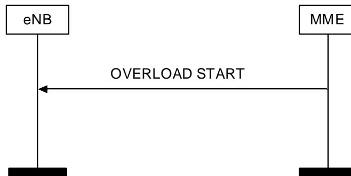
Figure 8.7.6.2-1: Overload Start procedure
