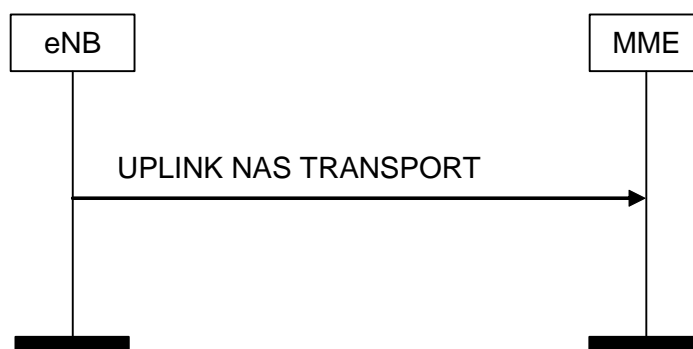
Figure 8.6.2.3-1: UPLINK NAS TRANSPORT Procedure
