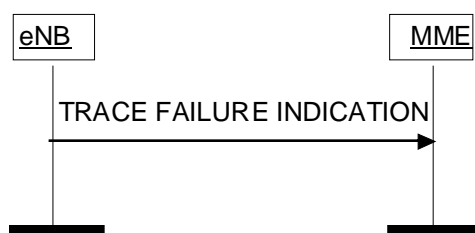
Figure 8.10.2.2-1: Trace Failure Indication procedure.
