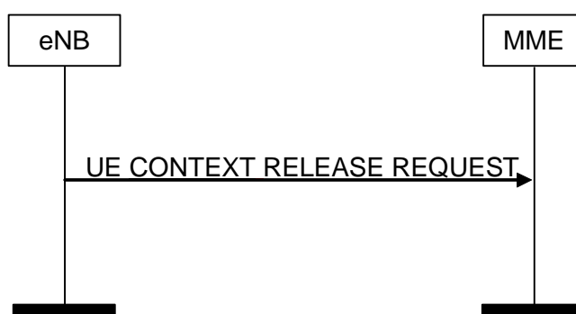
Figure 8.3.2.2-1: UE Context Release Request procedure. Successful operation.
