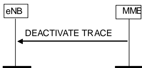
Figure 8.10.3.2-1: Deactivate Trace procedure. Successful operation.
