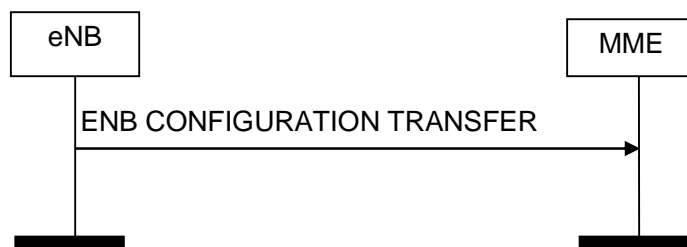
Figure 8.15.2.1-1: eNB Configuration Transfer procedure. Successful operation.
