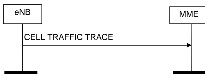
Figure 8.10.4.2-1: Cell Traffic Trace procedure. Successful operation.
