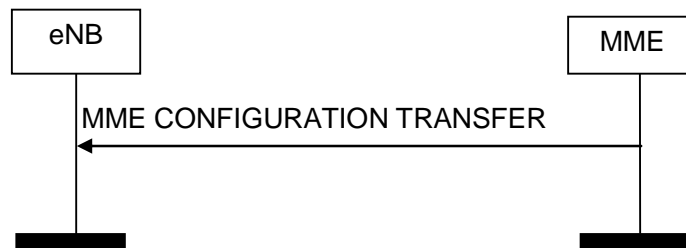
Figure 8.16.2.1-1: MME Configuration Transfer procedure. Successful operation.
