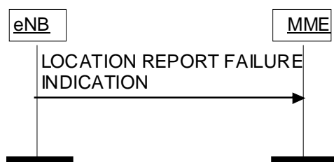
Figure 8.11.2.2-1: Location Report Failure Indication procedure.
