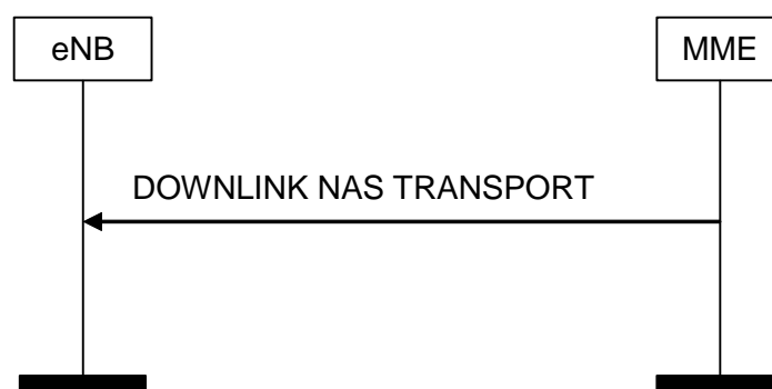
Figure 8.6.2.2-1: DOWNLINK NAS Transport Procedure
