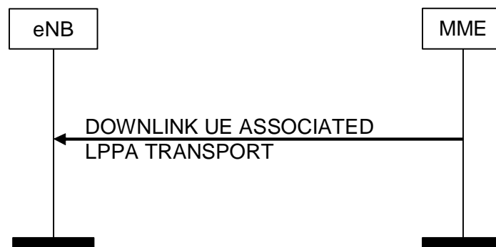
Figure 8.17.2.1-1: DOWNLINK UE ASSOCIATED LPPA Transport Procedure
