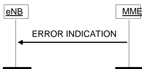
Figure 8.7.2.2-1: Error Indication procedure, MME originated. Successful operation.
