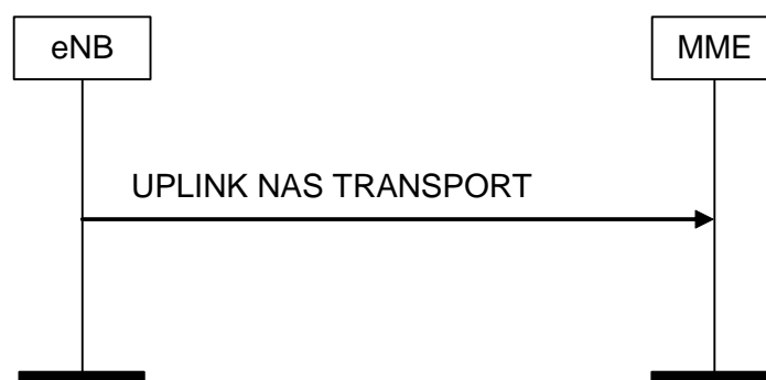
Figure 8.6.2.3-1: UPLINK NAS TRANSPORT Procedure
