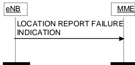
Figure 8.11.2.2-1: Location Report Failure Indication procedure.
