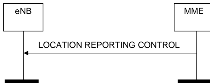
Figure 8.11.1.2-1: Location Reporting Control procedure. Successful operation.
