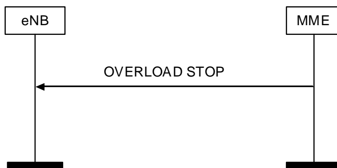
Figure 8.7.7.2.-1: Overload Stop procedure
