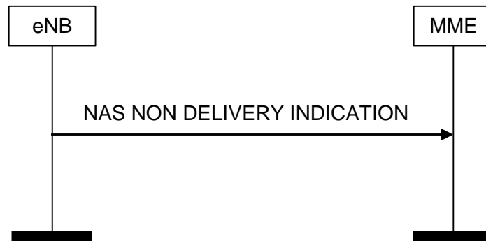
Figure 8.6.2.4-1: NAS NON DELIVERY INDICATION Procedure
