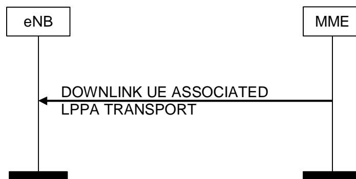
Figure 8.17.2.1-1: DOWNLINK UE ASSOCIATED LPPA Transport Procedure
