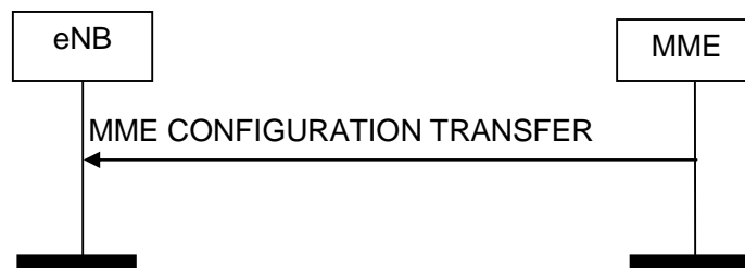
Figure 8.16.2.1-1: MME Configuration Transfer procedure. Successful operation.
