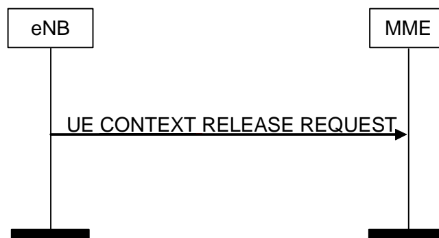
Figure 8.3.2.2-1: UE Context Release Request procedure. Successful operation.
