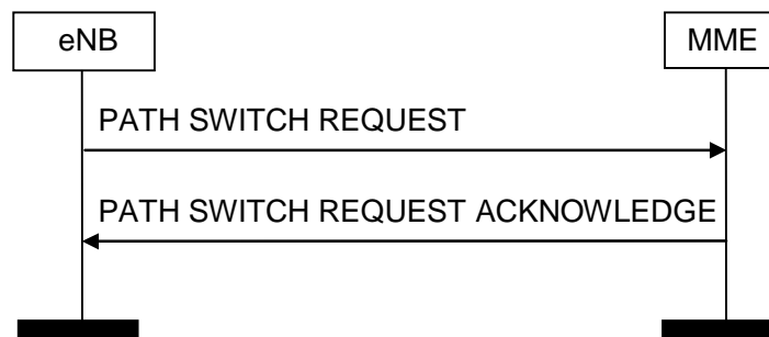
Figure 8.4.4.2-1: Path switch request: successful operation
