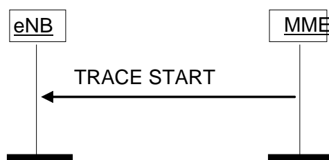
Figure 8.10.1.2-1: Trace Start procedure.
