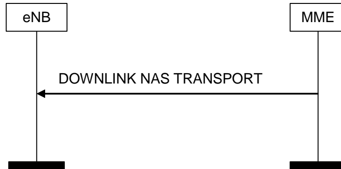
Figure 8.6.2.2-1: DOWNLINK NAS Transport Procedure
