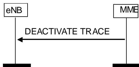
Figure 8.10.3.2-1: Deactivate Trace procedure. Successful operation.
