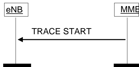
Figure 8.10.1.2-1: Trace Start procedure.
