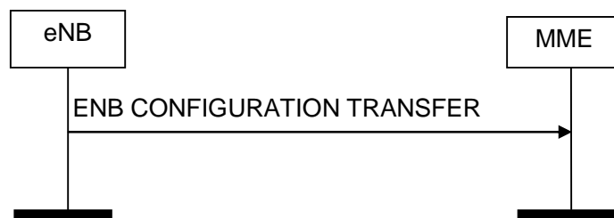
Figure 8.15.2.1-1: eNB Configuration Transfer procedure. Successful operation.
