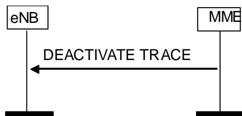
Figure 8.10.3.2-1: Deactivate Trace procedure. Successful operation.
