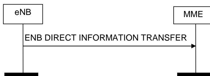
Figure 8.13.1.2-1: ENB Direct Information Transfer procedure. Successful operation.
