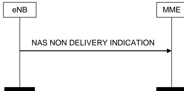
Figure 8.6.2.4-1: NAS NON DELIVERY INDICATION Procedure
