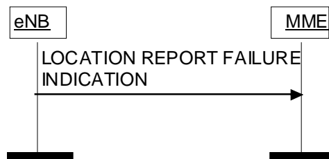
Figure 8.11.2.2-1: Location Report Failure Indication procedure.
