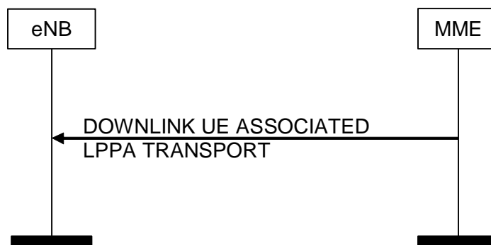
Figure 8.17.2.1-1: DOWNLINK UE ASSOCIATED LPPA Transport Procedure
