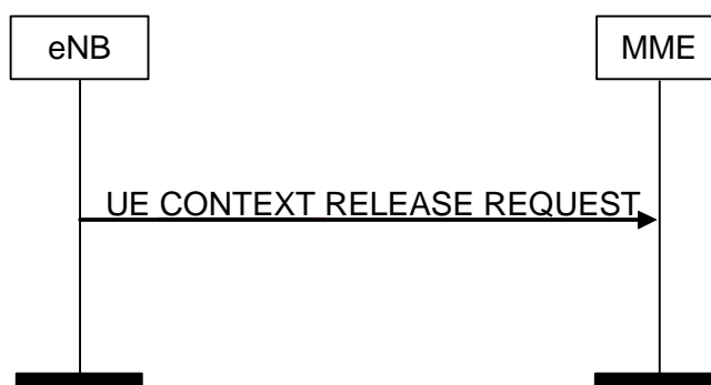
Figure 8.3.2.2-1: UE Context Release Request procedure. Successful operation.
