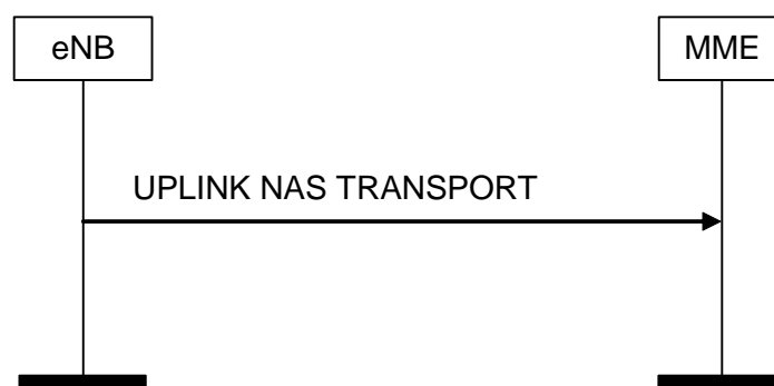
Figure 8.6.2.3-1: UPLINK NAS TRANSPORT Procedure
