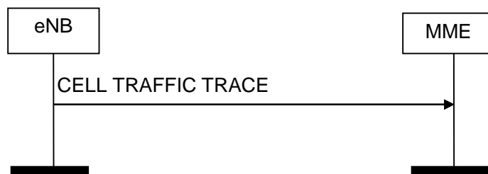
Figure 8.10.4.2-1: Cell Traffic Trace procedure. Successful operation.
