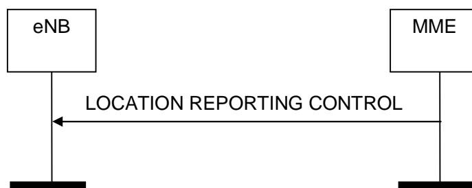
Figure 8.11.1.2-1: Location Reporting Control procedure. Successful operation.
