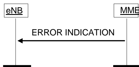
Figure 8.7.2.2-1: Error Indication procedure, MME originated. Successful operation.
