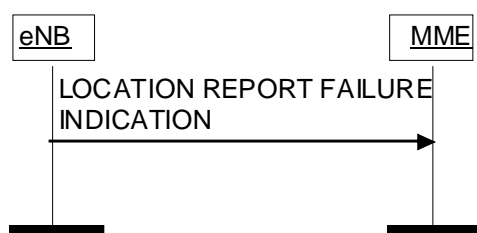
Figure 8.11.2.2-1: Location Report Failure Indication procedure.
