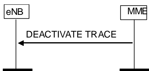
Figure 8.10.3.2-1: Deactivate Trace procedure. Successful operation.
