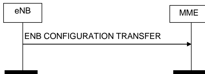
Figure 8.15.2.1-1: eNB Configuration Transfer procedure. Successful operation.
