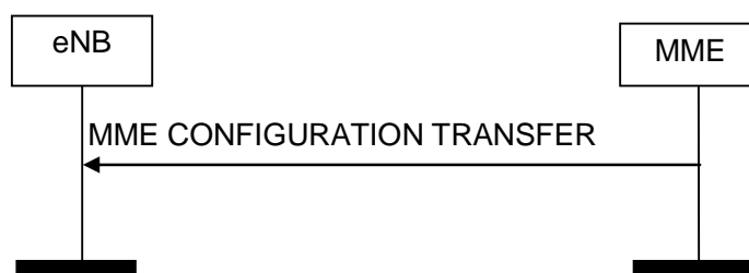
Figure 8.16.2.1-1: MME Configuration Transfer procedure. Successful operation.
