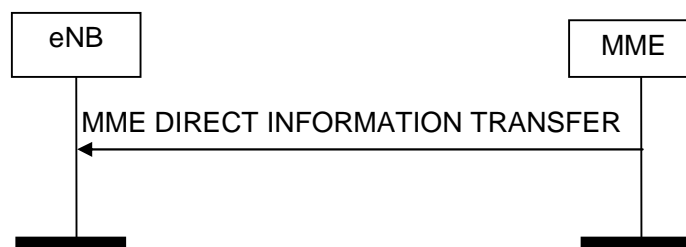
Figure 8.14.1.2-1: MME Direct Information Transfer procedure. Successful operation.
