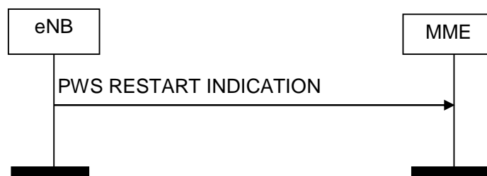
Figure 8.12.3.2-1: PWS Restart Indication procedure. Successful operation.
