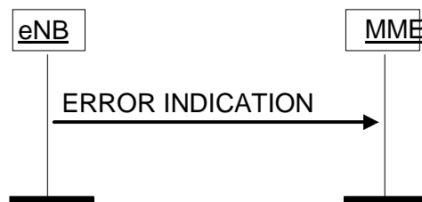
Figure 8.7.2.2-2: Error Indication procedure, eNB originated. Successful operation.
