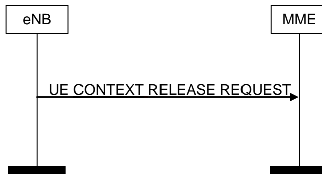
Figure 8.3.2.2-1: UE Context Release Request procedure. Successful operation.
