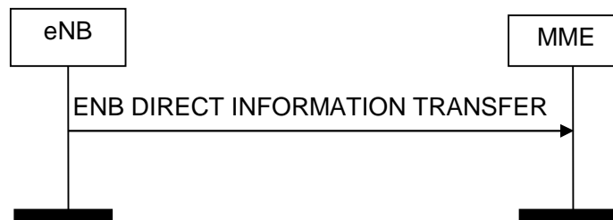
Figure 8.13.1.2-1: ENB Direct Information Transfer procedure. Successful operation.
