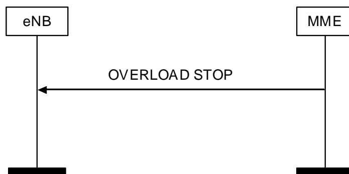
Figure 8.7.7.2.-1: Overload Stop procedure
