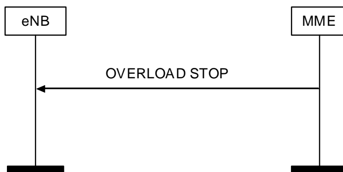
Figure 8.7.7.2.-1: Overload Stop procedure
